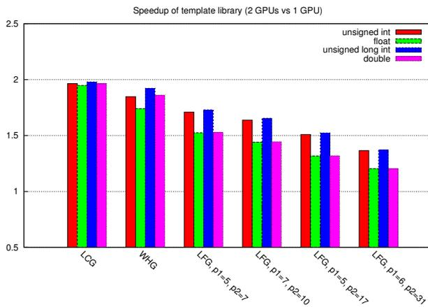
Fig. 6. Our template library: speedup 2 GPUs vs 1 GPU
