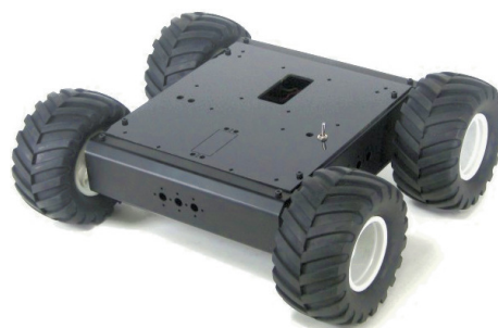
Fig. 1. Designed robotic platform based on A4WD1 chassis.
