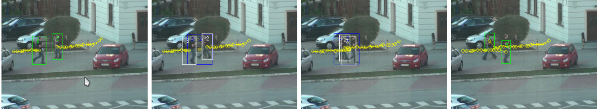
Fig. 2. Sample tracking sequence, green boxes - tracked pedestrians, white boxes - estimated pedestrians positions, blue boxes - group position, yellow circles - trajectories
