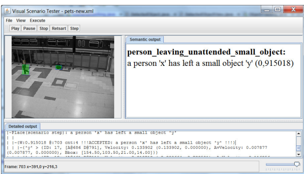
Fig. 9. Visual scenario tester. The displayed video frame and messages correspond to the place leave(isStill(y) \wedge atUnattendedDist(x,y)) of the FSPN specifying luggage left scenario.
