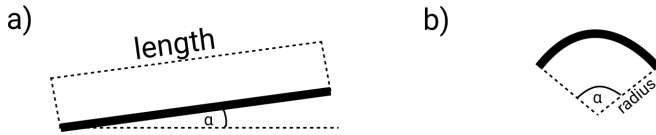
Fig. 2. The attributes used for line segments (a) and arches (b).
