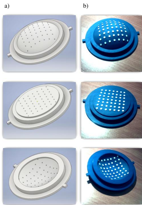
Fig. 8 Designed (a) and produced (b) model membrane shapes in 3D printing technology
