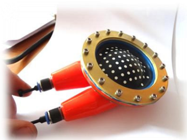
Fig. 2 Currently used proprietary ventricular assist pump model created using 3D printing (2017)
