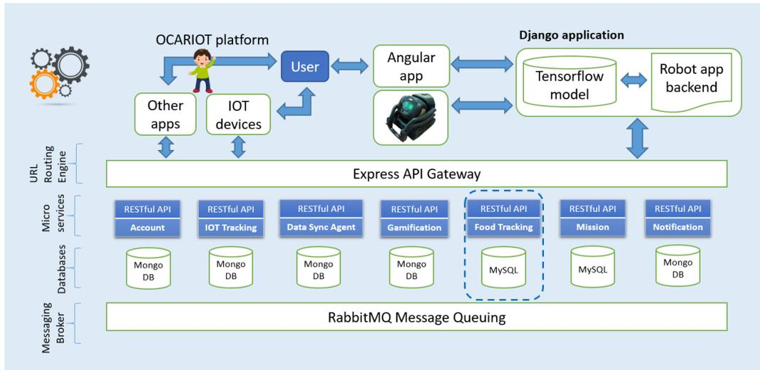
Fig. 4. Fruit Recognizing Social Robot integrated to OCARIoT
