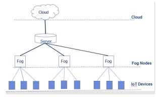
Fig. 2. Proposed security analysis model on Fog - IoT
