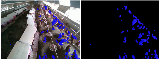
Fig. 6. Left: A single frame from a video recording from the farm. Right: The motion mask produced by MOG2.
