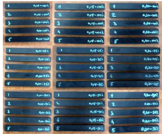
Fig. 3. 3-point bending specimens additively manufactured from rASA filament.
