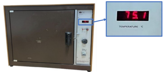
Fig. 3. Electrical convection oven ATS FAAR S110 FTE/D, used for heat treatment of tensile specimens made of PETG filament.
