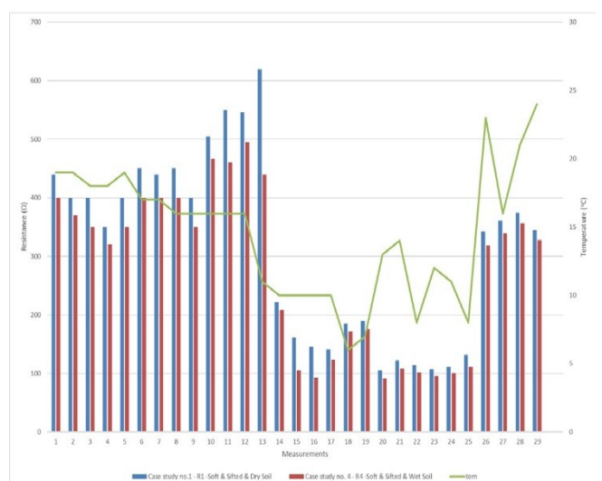
Figure 9. Ground Moisture effect on Grounding Resistance
