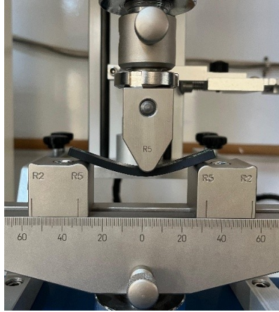
Fig. 4. 3-point bending test on the Barrus White 20 kN machine.
