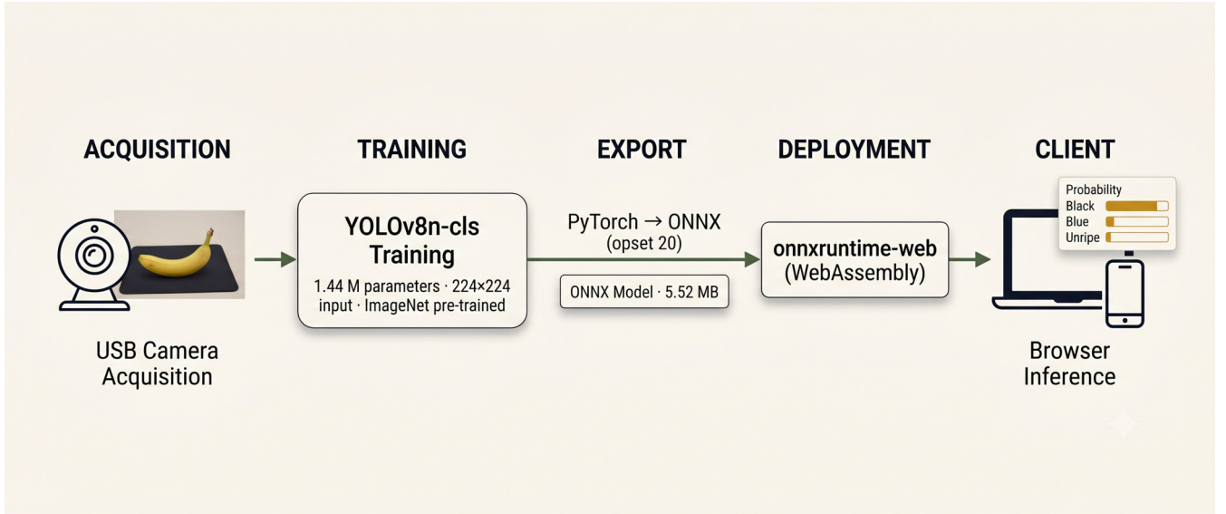
Fig. 1. End-to-end pipeline. Bananas are imaged with a USB camera, used to train a YOLOv8n-cls classifier, exported to ONNX, and deployed through onnxruntime-web for client-side inference inside any modern browser. No server component is required at inference time.
