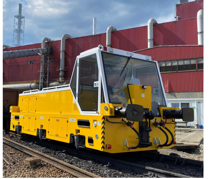
Fig. 1. ES3000 battery-electric shunting locomotive at an industrial site. A Teltonika FMB GPS tracker (roof-mounted) streams telemetry to the Wialon platform at 10-second intervals.
