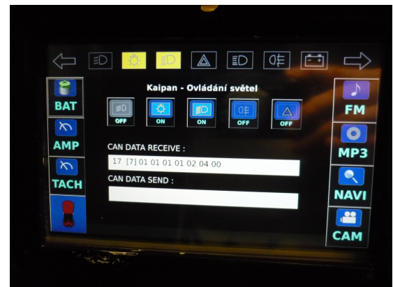
Fig. 4 LCD touch panel with QT embedded car system
