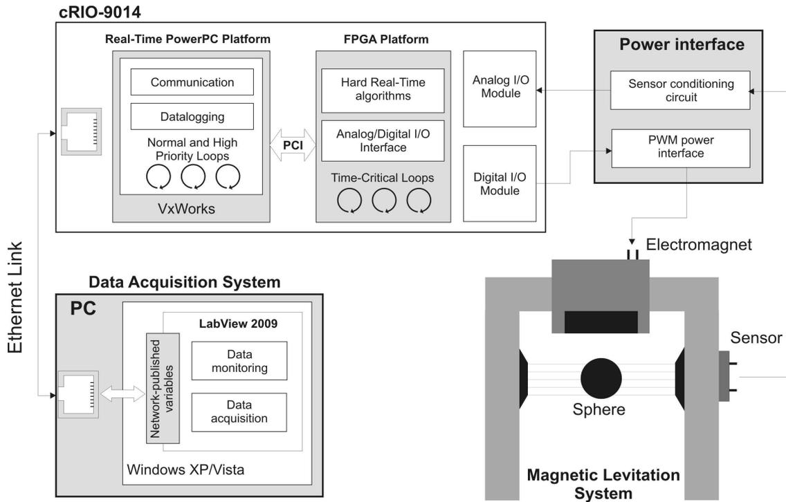
Fig. 1. Structure of magnetic levitation control system
