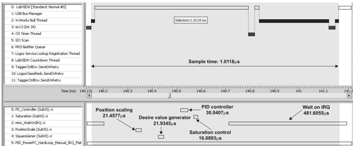
Fig. 5. Real-Time Execution Trace Toolkit session for the Power PC Interrupt ReQuest configuration with 1 ms sample period
