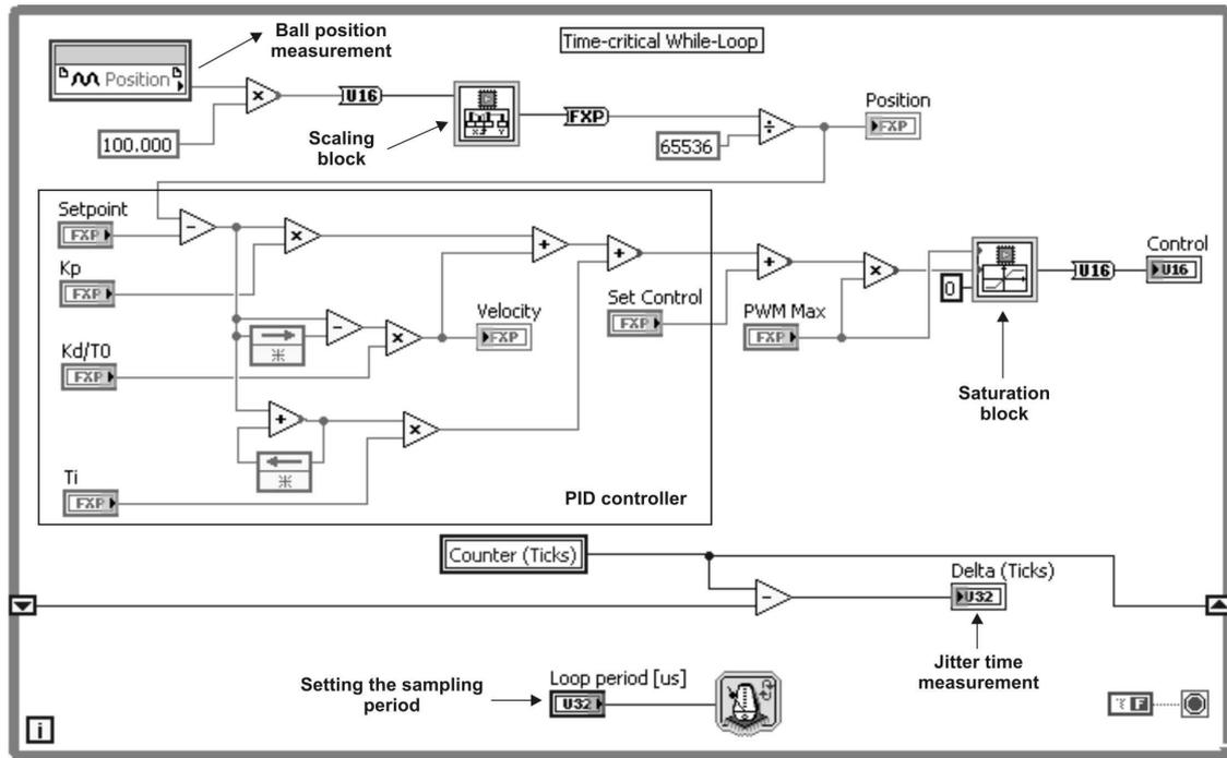
Fig. 3. The PID controller operating in a hard real-time loop running on FPGA chip
