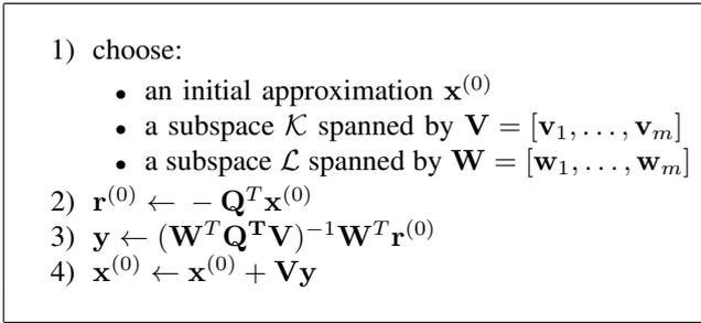
Fig. 1. A basic projection step for the equation  $\mathbf{Q}^T \mathbf{x} = \mathbf{0}$
