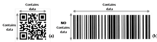
Fig. 1. Dimension for storing data in 2D (a) e 1D (b) codes
