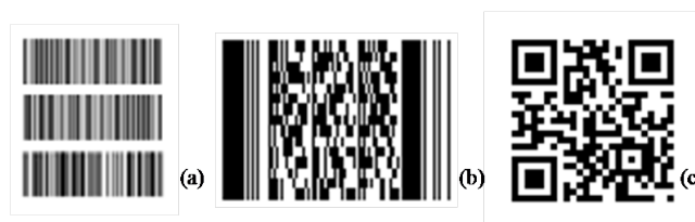
Fig. 2. Evolution of barcodes: multiple barcode layout (a), stacked barcode layout (b) and matrix barcode layout (c)
