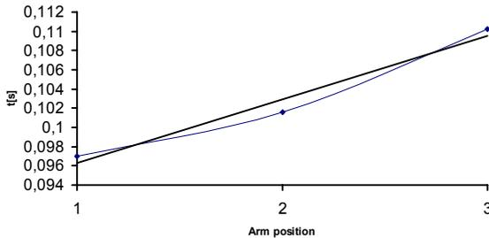
Fig. 11. Time delay between the starting point of the impedance signal measured on the thorax, and the starting point of  $\Delta Z_w$  as measured at the wrist, for three positions of the arm: (1) arm hanging freely down the body, (2) arm kept at the level of the heart, and (3) arm hold straight above head.
