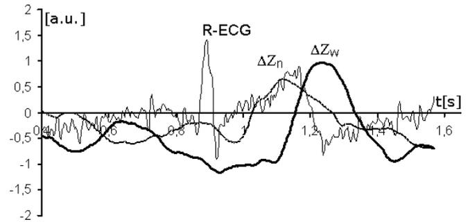
Fig. 7. One cycle of the signals presented in Fig. 6.  $\Delta Z_n$  denotes the impedance change recorded on the upper part of thorax, while  $\Delta Z_w$  is the impedance change recorded at the wrist. The hand was kept hanging down.
