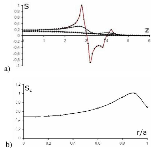
Fig. 4. Local sensitivity function (a) for conductivity changes at 0.5R (filled triangles), 0.9R (crosses) and 0.99R (filled squares), where R is the radius of the cylinder and b) total sensitivity,  $S_c$ , calculated as the sum (integral) of sensitivity S along coordinate "z" for different value of r. An anisotropic model, with anisotropy ratio equal to 2, was assumed.
