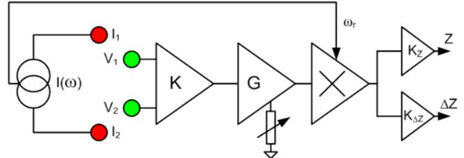
Fig. 1. Schematic diagram of measurement circuit,  $I(\omega)$  – current source,  $K$ ,  $G$ ,  $K_Z$ ,  $K_{\Delta Z}$  – gain of respective stage of bandpass amplifier, mark  $\times$  stands for synchronous demodulator
