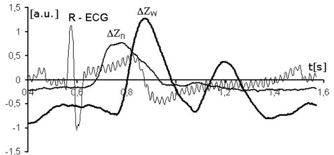
Fig. 8. One cycle of recorded signals with the hand kept at the level of the heart,  $\Delta Z_n$  denotes the impedance change recorded on the upper part of thorax, while  $\Delta Z_w$  is the impedance change recorded at the wrist.
