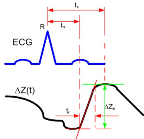
Fig. 3. Definition of time parameters and amplitude of the signal:  $t_n$ , the time delay between R wave in the ECG and the beginning of impedance signal  $\Delta Z_e$ ,  $t_x$ , the time delay between the R wave and the maximum of impedance signal  $\Delta Z_e$ , and  $t_r$ , the rise time of the signal.
