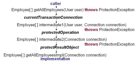
Fig. 5. Schematic view of the enriched getAllEmployees() method, the arguments and the return type of each generated part (if they were separate methods) and the implementation method.
