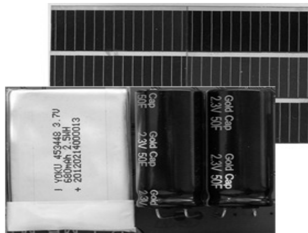
Fig 2. Solar cells (6 pcs. 29.4x12.3mm-40mW@1000W/m 2 ), rechargeable battery (Li-Pol: E=9057J) and super-capacitors (2x50 F/2.3V: E=264J)
