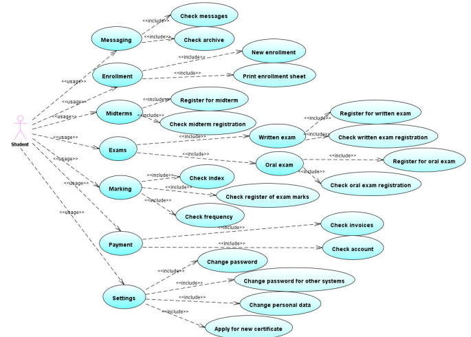
Fig. 3. A use case diagram for user role ‘student’ obtained by reverse engineering of e-Student (the leaves of the tree represent the functions this particular user role can perform).
