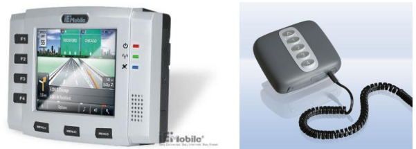
Fig. 5 a) Vehicle computer IET VTT-1000, b) Toll OBU
