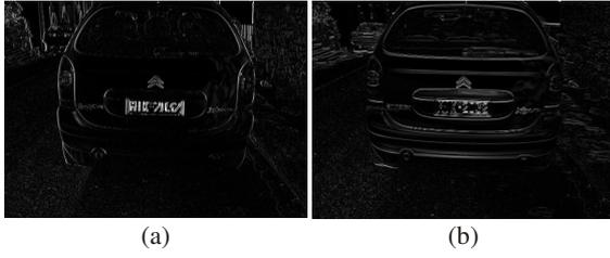
Fig. 2 Vertical (a) and horizontal (b) edge detection
