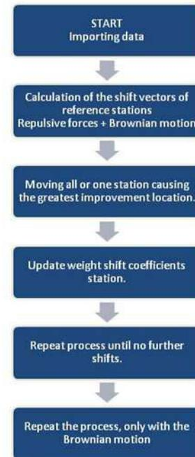
Fig. 4. Reference stations placement optimization algorithm.
