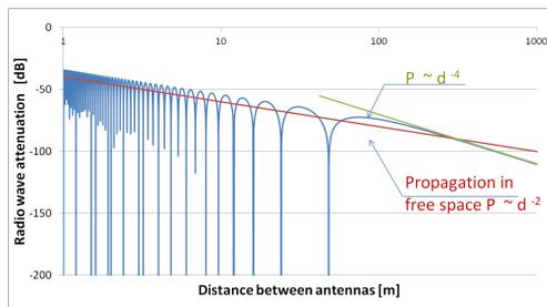
Fig. 2. Signal attenuation as a function of transmitter and receiver antennas separation
