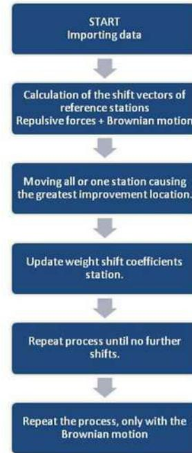
Fig. 4. Reference stations placement optimization algorithm.
