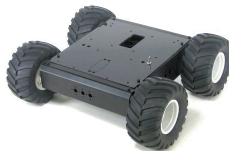
Fig. 1. Designed robotic platform based on A4WD1 chassis.
