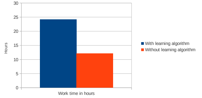
Figure 3. Difference in power consumption for device with and without learning algorithm implemented, with speed threshold set to 5km/h.
