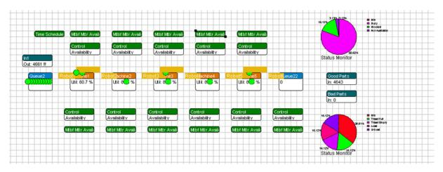
Fig. 5 Model of robotic line with failures after 8 hours of simulation
