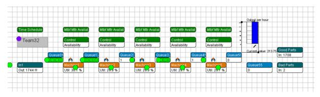
Fig. 4 Model of manually-operated line after 8 hours of simulation
