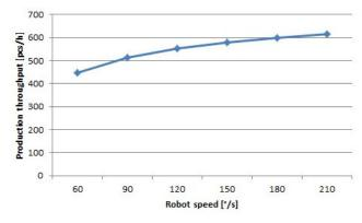
Fig. 3 Relation between productivity of robotic line and robot speed
