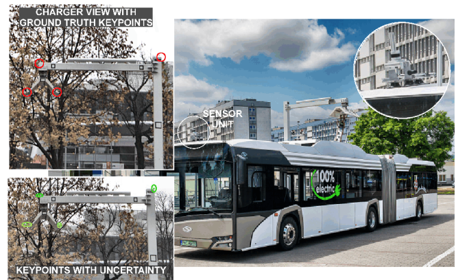
Fig. 1. Accurate detection of keypoint features for vision-based localisation of an electric bus while docking to a charging station. The inset images show a charging station with the ground truth keypoints (upper), the estimated locations of these keypoints with uncertainty ellipses (lower), and a close-up of the roof-mounted sensor unit with a camera (in the circle)
