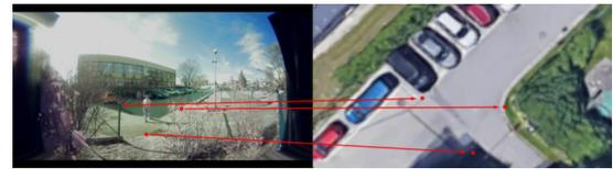
Figure 3: A photo showing the process of calculating the homography matrix. The person responsible for the configurations marks the points on the image from the camera and the corresponding 2D map.
