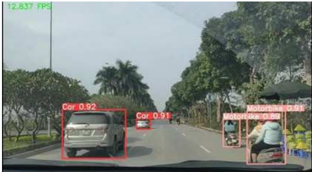
Figure 13: Identification results using Dashcam YOLO v5 model.
