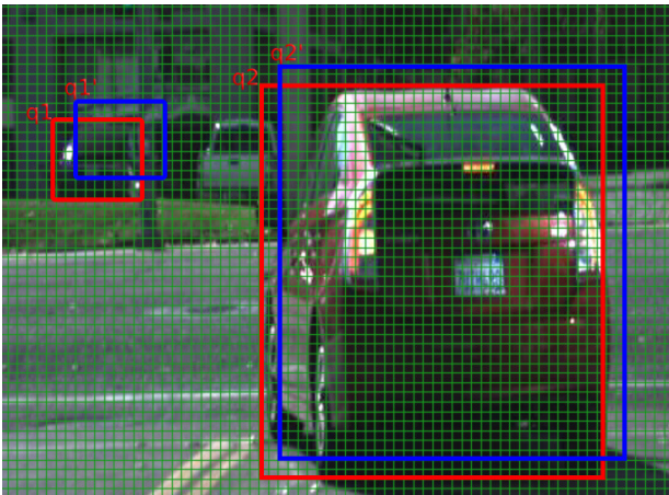
Fig. 1: By naively dividing an image in 255x255 grid quantization range (green lines), vertices q_1 and q_1' are different by two quantized values. Same for q_2 and q_2' . The detection between 2 close quantized values can affect differently on the final result based on the different scales of objects in an image
