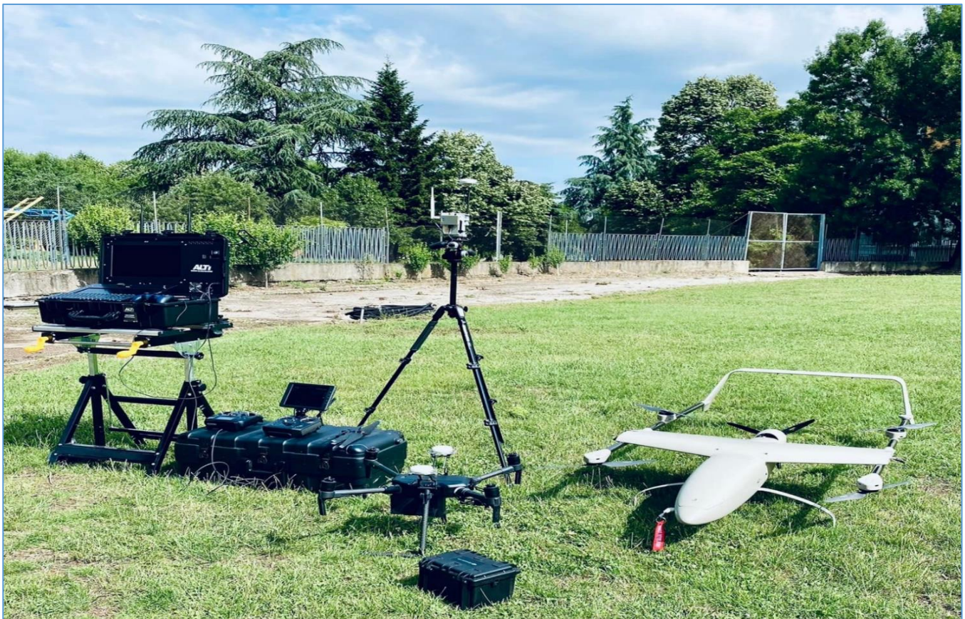
Fig.3. The UAVs used in the THEASIS-M system for early detection and monitoring of wildfires – (from left to right) the ground control station of the ALTi Transition F, the DJI Matrice M210 RTK drone with its case, remote controller and RTK station and the ALTi Transition F with its wings removed.
