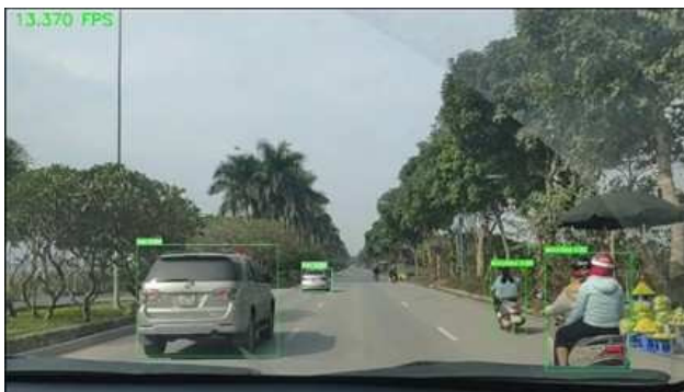
Figure 14: Identification results using Dashcam YOLO v7 model.
